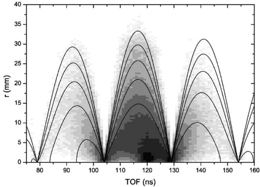
**Figure 8.** The electron radial displacement  $r$  on the detector versus the electron TOF for single ionization of  $H_2$  by 6 MeV proton impact. The cyclotron revolution time corresponds to a magnetic field strength of 14 Gauss. The solid lines are the calculated displacements  $r$  for electrons with kinetic energies between 10 and 50 eV in steps of 10 eV. The point (TOF = 120 ns,  $r = 0$ ) represents the origin ( $E_e = 0$ ) on the electron energy scale (from Moshhammer *et al* (2003b)).
