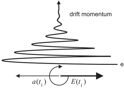
FIG. 1. Trajectory of an electron with zero initial momentum ionized at time  $t_i$  by a clockwise-rotating circularly polarized laser pulse. The pulse propagation direction is directed into the page. The asymptotic direction of the electron drift momentum  $\vec{p}_{\text{end}}$  is perpendicular to that of the electric field  $\vec{E}(t_i)$  and its acceleration  $\vec{a}(t_i)$  at the instant of ionization.
