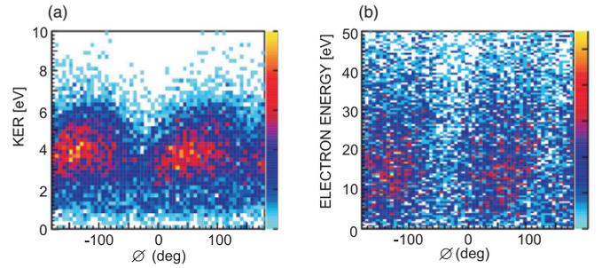
FIG. 15. (Color online) Dependence of the dissociative ionization rate on the angle between the electron momentum vector and the internuclear axis in the polarization plane and on (a) the KER and (b) the energy of the tunnel electron. Laser intensity  $I \approx 6 \times 10^{14}$  W/cm<sup>2</sup>.
