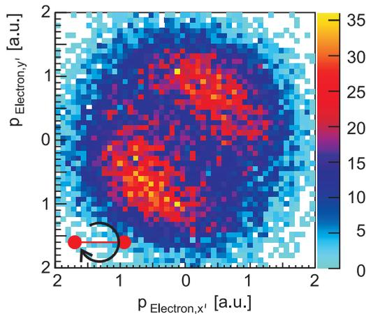
FIG. 11. (Color online) Electron momentum distribution in the molecular frame projected onto the polarization plane for 40-fs,  $6 \times 10^{14} \text{ W cm}^{-2}$  circularly polarized laser pulses. The sense of rotation is clockwise, as indicated in the bottom left-hand corner. The molecular axis is orientated along the  $x'$  axis (from [18]).
