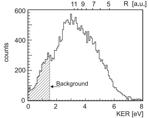
FIG. 7. KER distribution for linearly polarized laser pulses. Ascribed internuclear separations are shown at the top.
