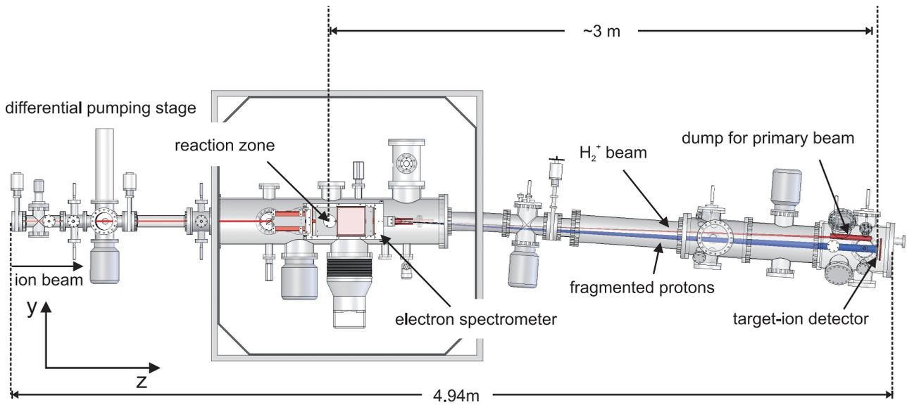
FIG. 3. (Color online) Overview of the experimental setup. The reaction zone, defined by the overlap of  $H_2^+$  and laser beams, is located inside the electron spectrometer, where a homogeneous electric field is applied. The target-ion detector is located at a distance of 3 m behind the reaction zone. Compensation for the earth's magnetic field is achieved by externally mounted Helmholtz coils.
