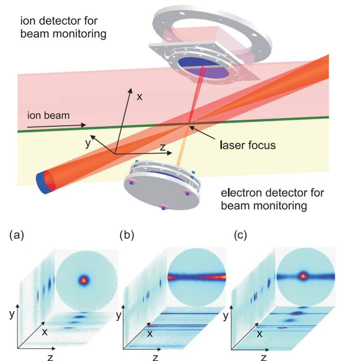
FIG. 5. (Color online) (top) Depiction of the beam-monitoring arrangement. Laser and ion beams produce ion-electron pairs which are guided to the monitoring detectors by an applied electric field. (bottom) Images produced by the beam monitoring system: (a) only laser beam present in reaction chamber, (b) only ion beam present in reaction chamber, and (c) both ion and laser beams present in the chamber.
