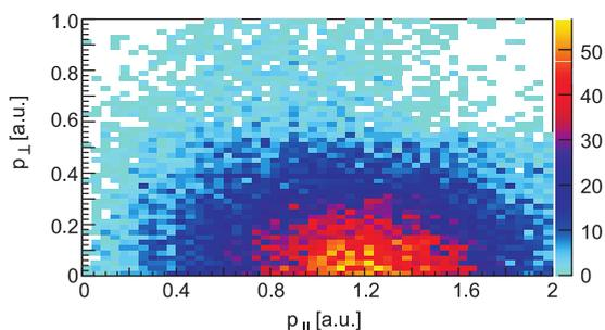
FIG. 12. (Color online) Electron momentum distribution showing the dependence of electron counts on the magnitude of the components of electron momenta within ( $p_{\parallel}$ ) and perpendicular to ( $p_{\perp}$ ) the polarization plane.
