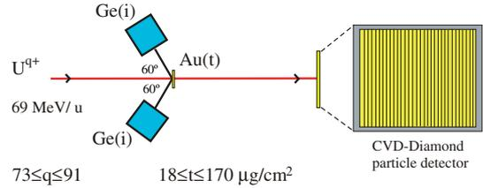
Fig. 1. The experimental set-up showing the Ge(i) X-ray detectors and the position sensitive CVD-diamond particle detector.
