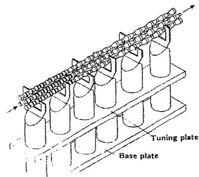
FIG. 3. Principle of the tunable four-rod RFQ structure.
