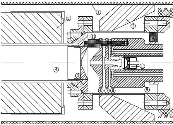
FIG. 1. Cross section through the electron-gun assembly in the extraction area of the Frankfurt ECRIS. (1) Main insulation pipe; (2) hexapole; (3) magnetic-field shaping plug (iron); (4) plasma chamber; (5) moveable plasma chamber electrode; (6) puller electrode; (7) anode; (8) Wehnelt cylinder (water cooled); (9) iron cylinder; (10) cathode with 3 mm hole; (11) insulators.
