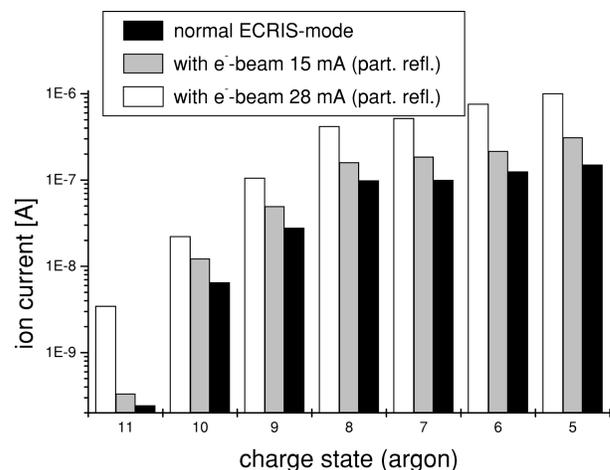
FIG. 3. Charge state spectra measured after use of the analyzing magnet for various conditions as indicated. The source voltage was 15 kV; all charge state spectra are recorded after optimizing the beam optics to transport the  $Ar^{8+}$  charge state.
