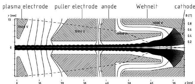
FIG. 2. IGUN simulation of the formation of the electron beam.
