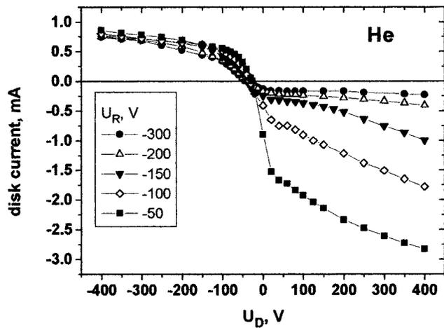
FIG. 1. Currents to the biased disk as a function of the disk voltage at different voltages at the biased ring. The ECR discharge is sustained in pure helium gas.
