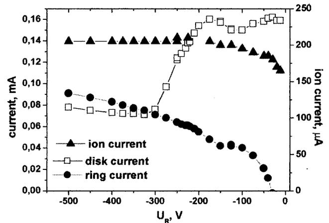
FIG. 2. Currents to the biased disk and to the biased ring (left scale) and ion currents to the Faraday cup (right scale) as a function of the ring voltage at a fixed biased disk voltage of  $-200$  V. The ECR discharge is sustained in pure argon gas. The ionic currents are measured in a Faraday cup directly in front of the magnet for charge-state analysis.
