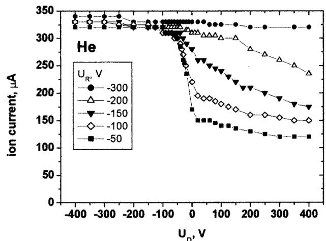
FIG. 3. Total ion currents (not charge state analyzed) from a He plasma as a function of the biased disk voltage at different settings of the biased ring voltages.
