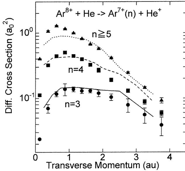
**Figure 3.** The differential cross section for the one-electron capture from He to  $n = 3-5$  states of  $\text{Ar}^{7+}$  as a function of  $p_{\perp R}$ . Symbols denote the experimental results and curves are the calculation results.
