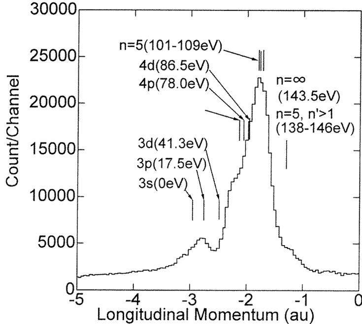
**Figure 1.** The longitudinal momentum distribution of the recoil ions for one-electron capture from He by  $0.25 \text{ MeV u}^{-1} \text{ Ar}^{8+}$  ions. The recoil-ion yield is integrated over the transverse momentum between 0 and 4 au. The electronic states of the captured electron and their excitation energies are also indicated.
