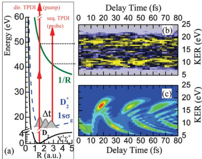
FIG. 1. (Color online) (a) Illustration of the dominant dissociative pathways for direct and sequential TPDI of  $D_2$ . (b) Density plot for the experimental KER spectrum of coincident  $D^+ + D^+$  fragments as a function of delay time up to 80 fs. (c) The same as (b), but for theoretical results.
