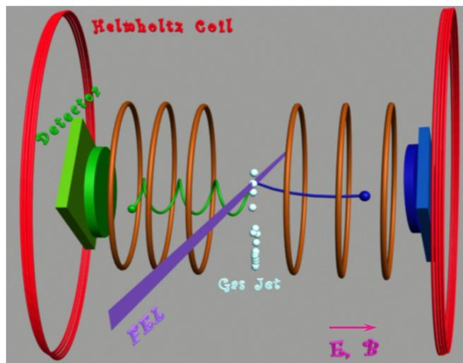
Figure 1. Schematic of a reaction microscope.
