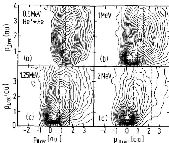
Fig. 1. Double differential cross sections for reaction (1). The y-axis shows the momentum of the recoiling  $\text{He}^+$  ion perpendicular to the beam axis and the x-axis the momentum in beam direction (positive value means forward emission). The long dashed line shows the estimated position of the (Ne) interaction.
