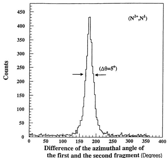
Fig. 8. The difference between the azimuthal angles of the first fragment  $\phi_1$  and second fragment  $\phi_2$  represented in the range from  $0^\circ$  to  $360^\circ$ .
