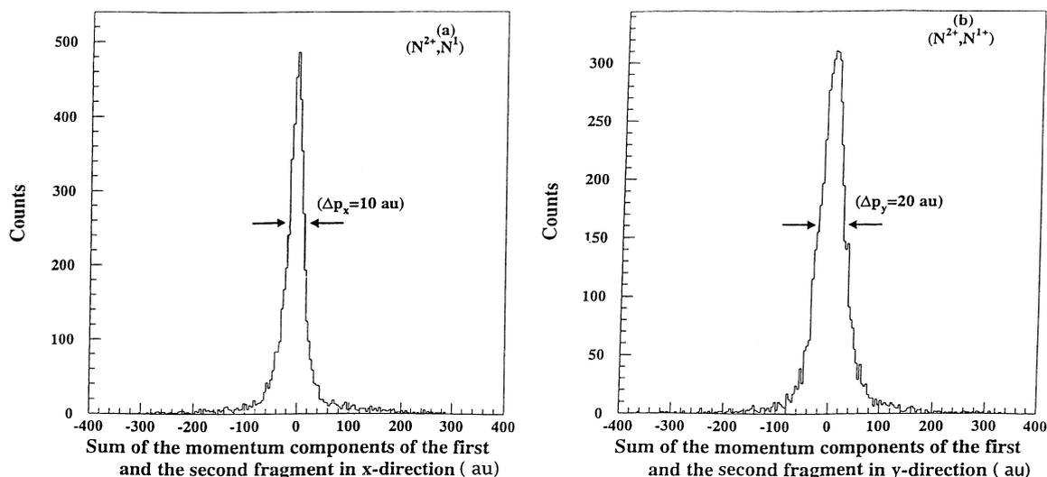
Fig. 9. The sum of the momentum components for both fragments derived from the TOF in the  $x$ -direction (a) and the position on the recoil ion detector (perpendicular to the beam direction) in the  $y$ -direction (b), respectively.
