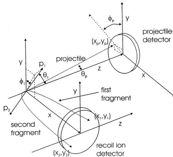
Fig. 4. Kinematics picture of the collision process where the momentum vectors of projectile, first recoil-ion and second recoil-ion are presented in Cartesian and spherical coordinates with the different measured momentum components and angles.
