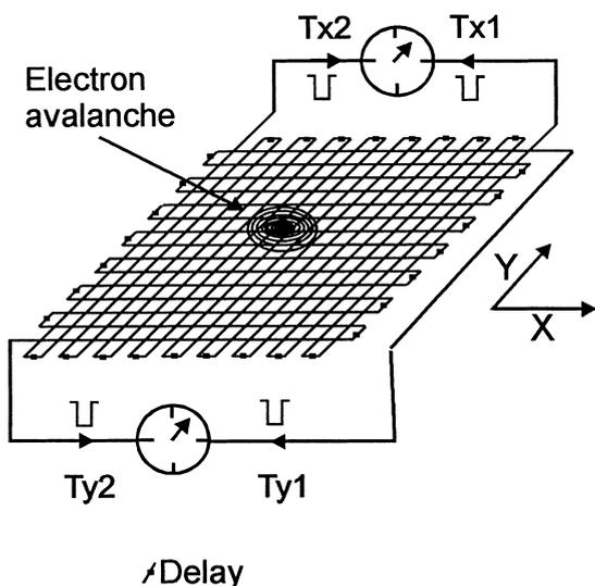
Fig. 2. Two position planes and the function principle of the delay-line-anode. The delays is obtained just from the length of the wire turns. The Clocks represent time measurements.
