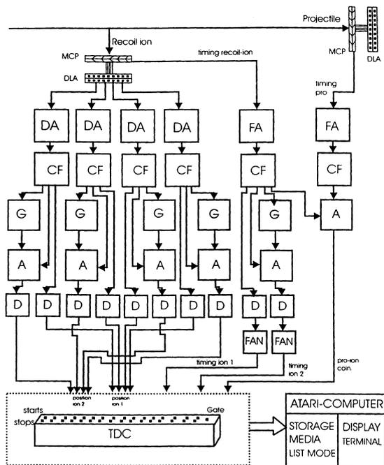
Fig. 3. Electronic set-up of the position-sensitive multi-hit-detector-system. The different shorts mean the following. DA: difference amplifier, CF: constant fraction, G: Gate and delay unit, A: coincidence module, FAN: Fan in/out module, D: cable delay and TDC: time to digital converter.
